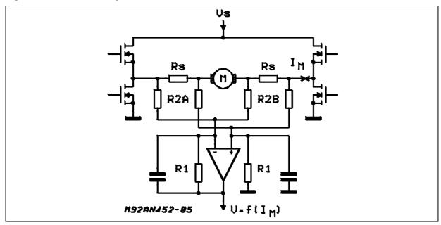
Fig. 5 shows another circuit that is feasible for all situations in which, since they cannot be inserted in the source circuit, the shunts have to be connected directly in series with the load, with all the disadvantages that this entails.
