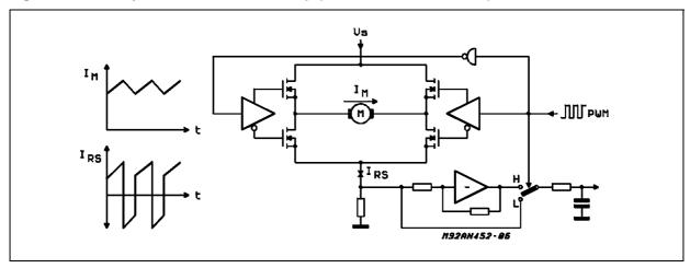
Figure 7. Accovery of the Load Current Map. (Inverting/non Inverting Solution)
