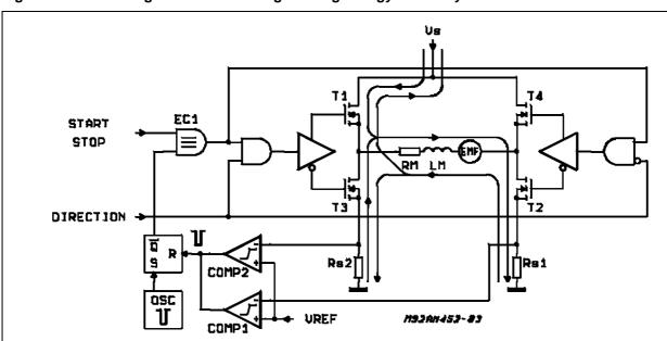
Figure 3. Same As Figure 1 but Including Braking Energy Recovery.
